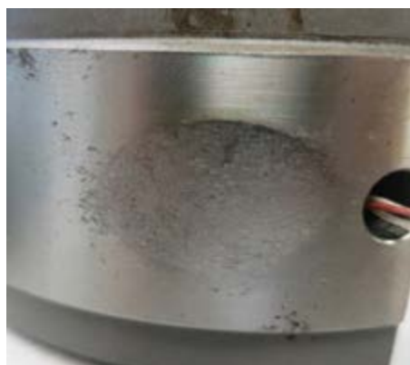
Figure 2: Pivot wear on the point-contact-pivot tilt pad (left) and bearing shell bore (right)
