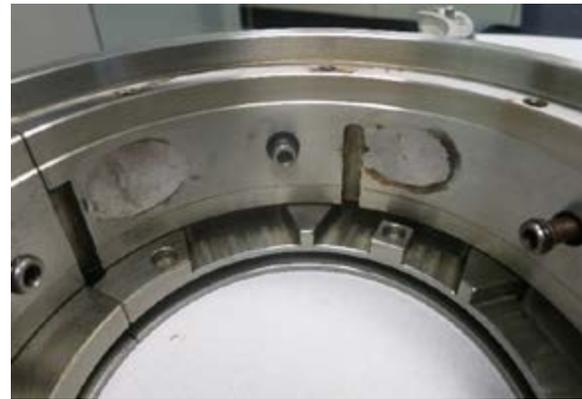
Figure 2: Pivot wear on the point-contact-pivot tilt pad (left) and bearing shell bore (right)
