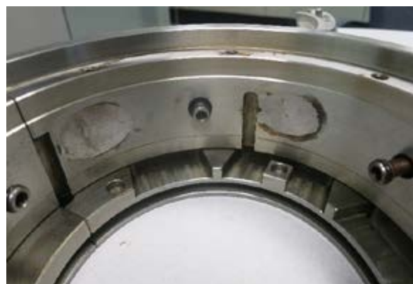
Figure 2: Pivot wear on the point-contact-pivot tilt pad (left) and bearing shell bore (right)
