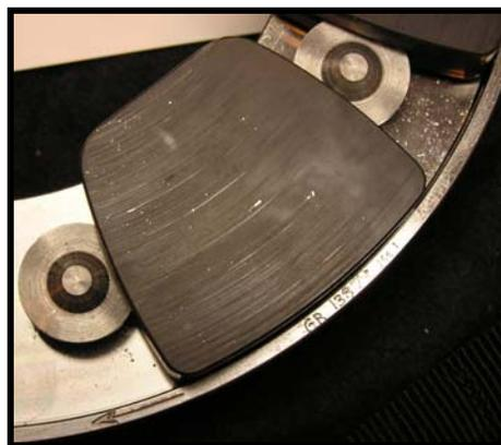
**Fig 4. Polymer Lined Thrust Bearing with Showing Embedded Metallic Debris**
