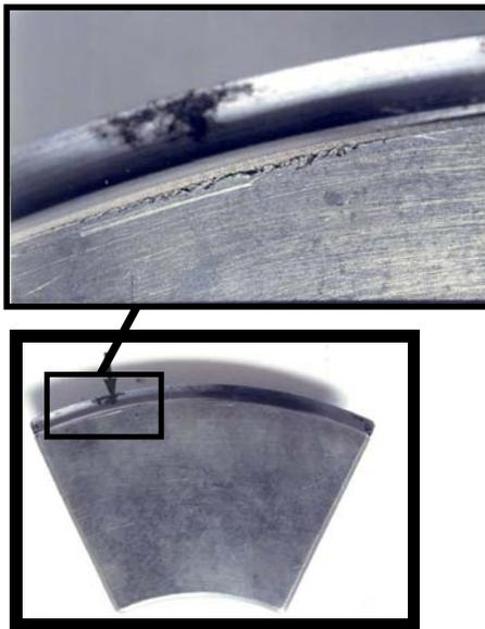
**Fig 24. Cavitation Damage on a Thrust Tilt Pad.**
