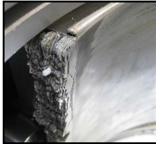
**Fig 35. Wiping of a Journal Tilt Pad
