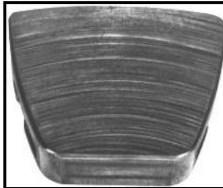
**Fig 2. Abrasive Damage due to Foreign Material During Operation.**
