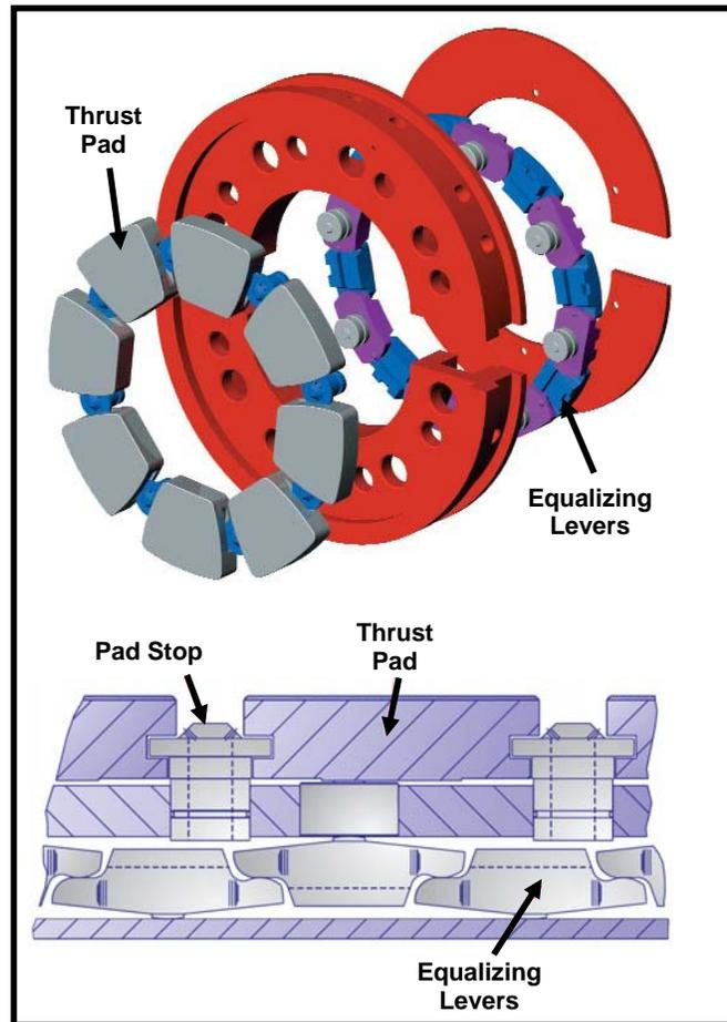
**Fig 32. CQ Leveling Mechanism for Tilt Pad Thrust Bearing.**
