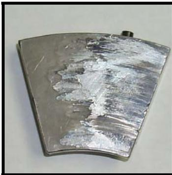
**Fig 16. Wiping of a Tilt Pad Thrust Bearing Due to Loss of Lubrication.**
