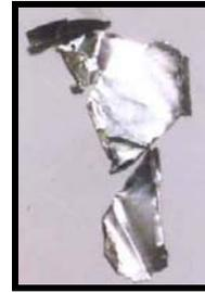
**Fig 19. Thin 'Foil' of Babbitt Removed from Pad in Figure 17.**
