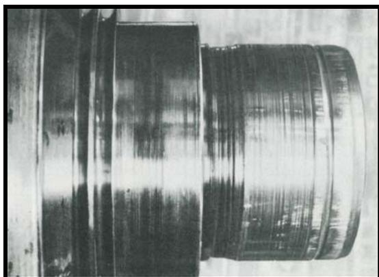
**Fig 5. Wire Wooling of Shaft.**
