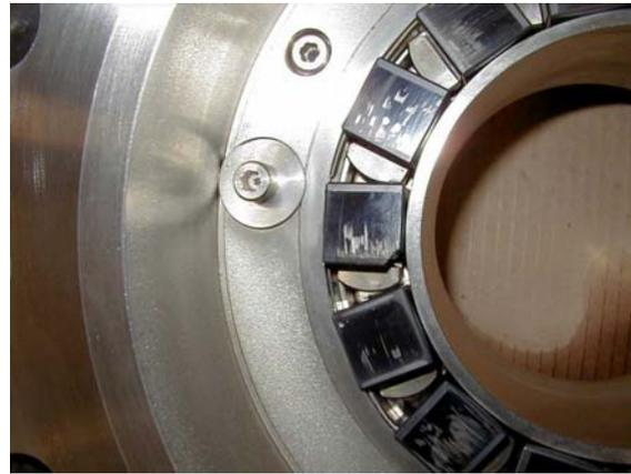
**Figure 37 Scuffing of Ceramic Thrust Pad Surfaces During Start-up and Shutdown.**
