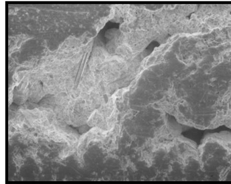
**Fig 25. Scanning Electron Micrograph of Cavitation Damage on the Edge of the Thrust Pad Shown in Figure 23.**
