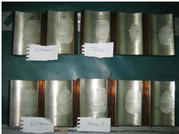
**Fig 21. Wiping of All Journal Tilt Pads Due to Loss of Clearance at Start-up.**
