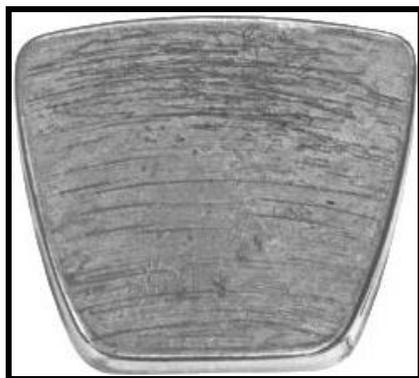
**Fig 1. Abrasive Damage due to Foreign Material at Start-Up.**
