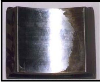
**Fig 18. Light Wiping of a Journal Tilt Pad Due to a Momentary Reduction in Oil Flow.**
