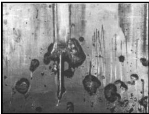
**Fig 3. 'Haloes' From Embedded Particle.**
