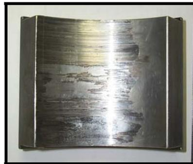
**Fig 17. Light Wiping of a Journal Tilt Pad Due to a Momentary Reduction in Oil Flow.**
