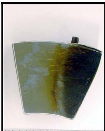
**Fig 10. Coking on Thrust Pad Due to Excessive Temperature.**
