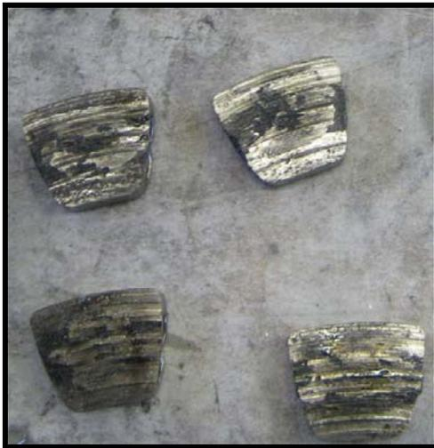
**Fig 8. Wiped Thrust Pad
