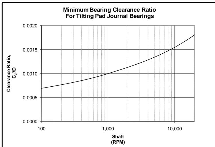
**Fig 23. Minimum Bearing Clearance as a Function of Speed**
