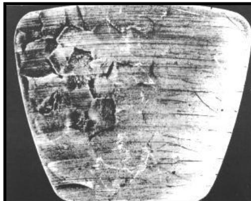
**Fig 11. Faceted Thrust Bearing Pad Due to Thermal Cycling of Pad.**
