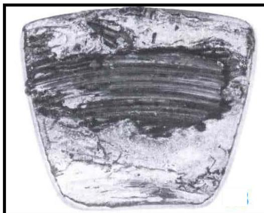
**Fig 6. Black Scab on Thrust Pad.**
