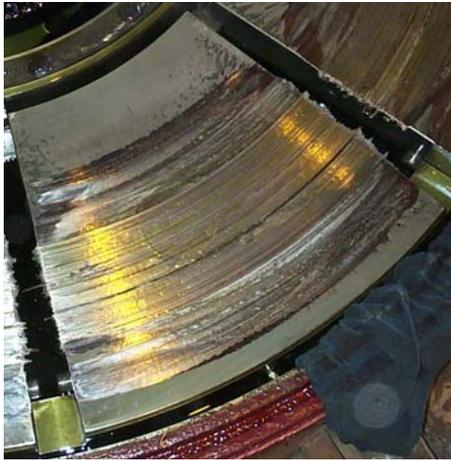
**Fig 36. Damaged Thrust Tilt Pad with a Hydrostatic Lift Pocket; Hydrostatic System Failed.**
