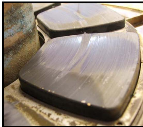
**Fig 9. Worn Polymer Thrust Pad**
