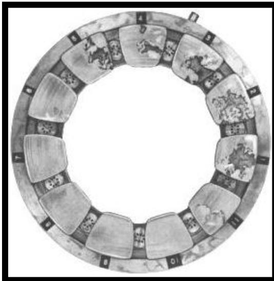
**Fig 31. Tilt Pad Thrust Bearing Damage Due to Misalignment.**
