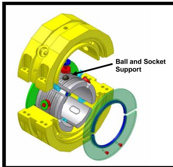
**Fig 33. Ball and Socket Support for Tilt Pad Journal Bearings.**
