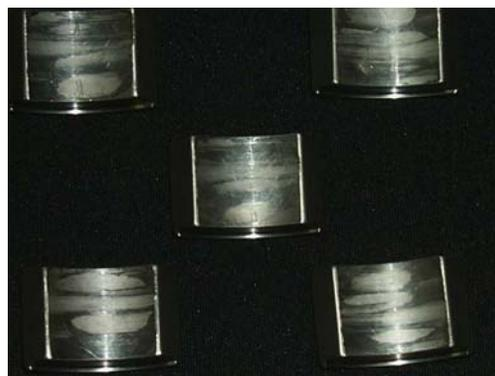
**Fig 22. High Dynamic Load Damage to All Tilt Journal Tilt Pads.**
