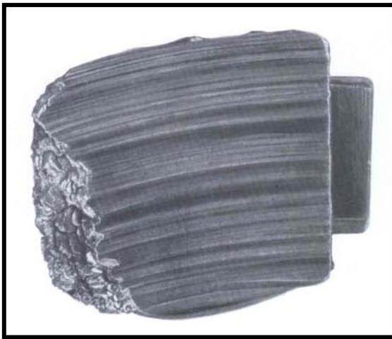
**Fig 34. Wiping of a Thrust Tilt Pad
