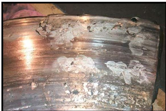
**Fig 12. Intergranular Cracking on a Thrust Pad From Excessive Temperatures.**
