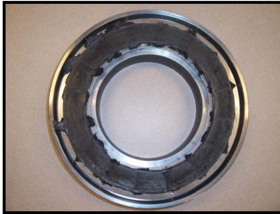
**Fig 20. Damaged Polymer Thrust Bearing Due to Insufficient Lubrication.**
