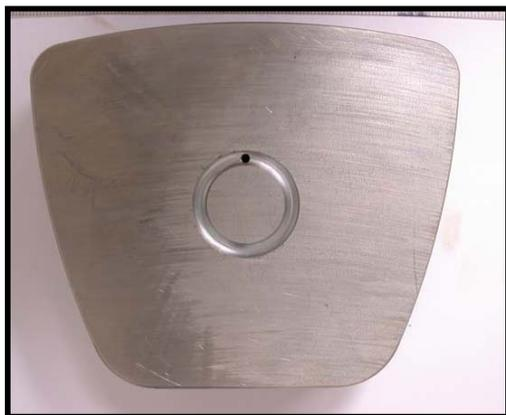
**Fig 26. Thrust Tilt Pad with Electrical Discharge Damage.**
