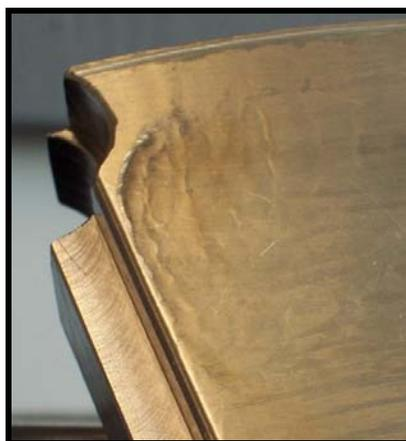
**Fig 13. Thrust Pad with Rippled Surface From Creep.**
