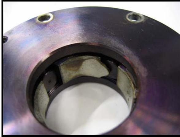
**Fig 14. Tilt Pad Journal Bearing Damaged by Heat Soak Back.**
