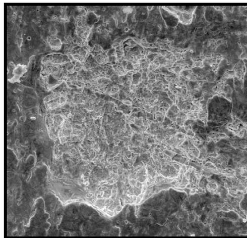
**Fig 29. Microphotograph of 'Pit' From Electrical Discharge; Smooth Features at Higher Magnification.**
