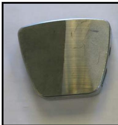
**Fig 27. Thrust Tilt Pad with Electrical Discharge Damage.**
