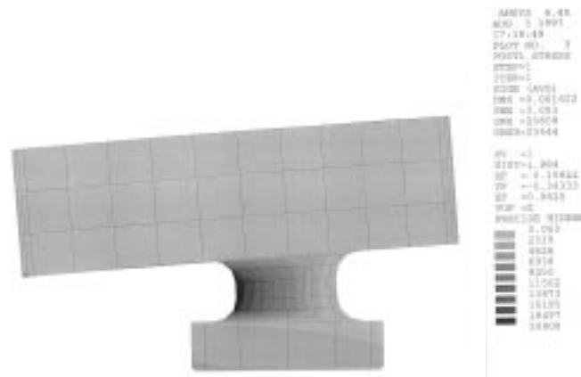
Figure 20. Exaggerated Deflection of the FP Pad and Stress Contours.
