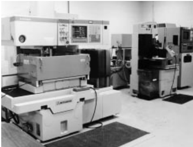
Figure 11. Wire EDM Machines Utilized in the Manufacture of FP Journal Bearings.
