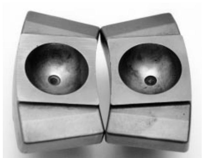
Figure 17. Pivot Wear on the Socket of the Upper Leveling Link.
