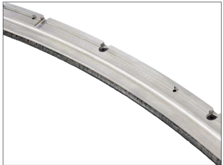
A brush seal generally consists of three components: a front plate, a back plate and a bristle pack, which bends with rotor contact to maintain low leakage.
