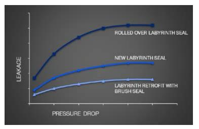
Brush seals can reduce leakage by up to 80%.
