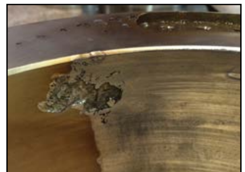
(Top to bottom) Severe wiping of thrust pad from inadequate lubrication; field analysis of bearing damage; babbitt fatigue.
